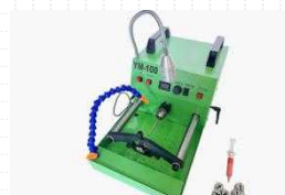
NO.1202 YM-100 Precision Horizontal Honing Machine, for grinding various denso valve rod
